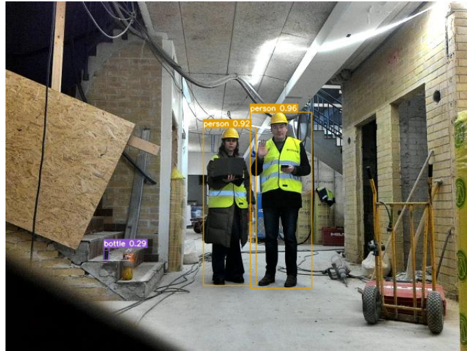
Figure 4.6: Example of a YOLOv7 model detecting objects in an image from Vipan.
