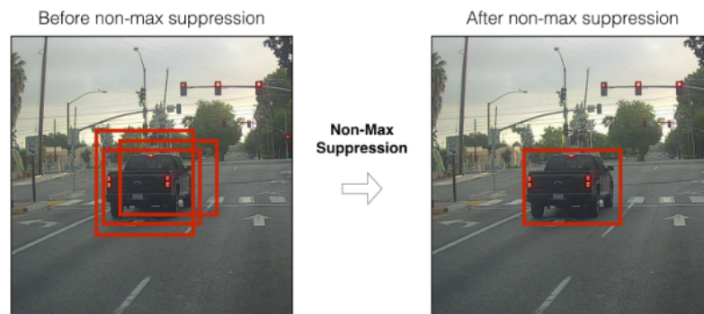
Figure 2.13: Example of the result using non-max suppression when detecting a car [?].
