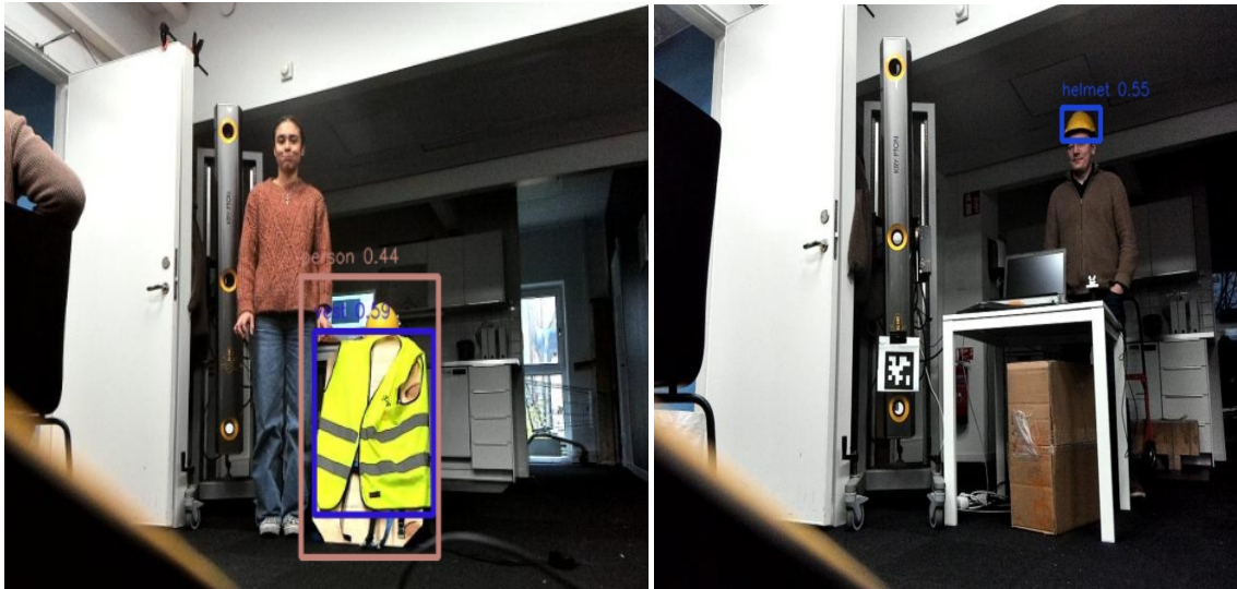
Figure 4.7: Example of an detection on Spot with the YOLOv7 model trained with the SODA dataset. The model fails to detect a person and detects a board with a vest as a person instead.
