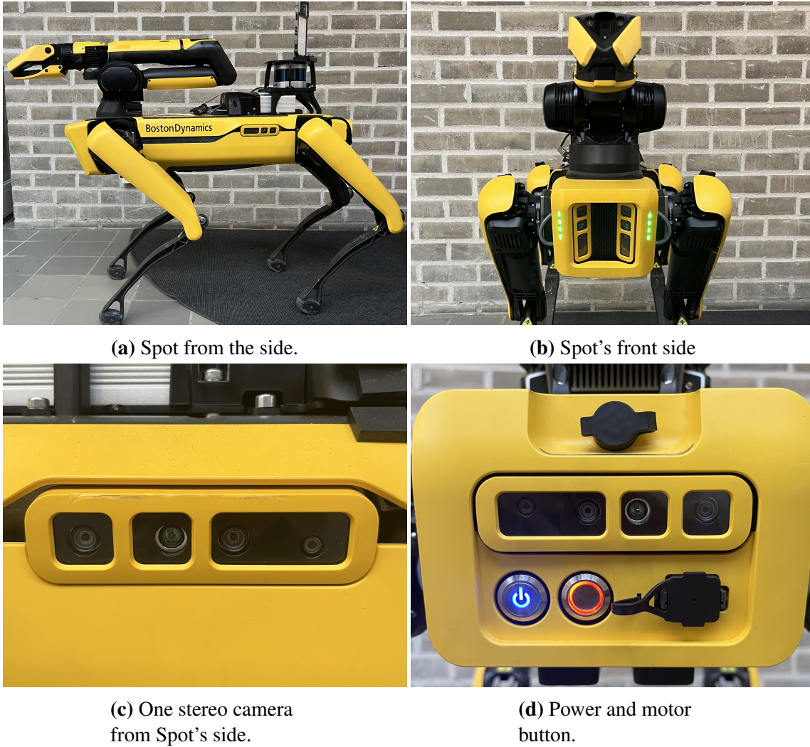
Figure 2.1: Figures of Spot and its hardware features.
