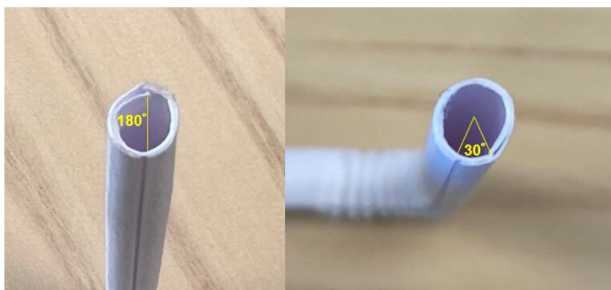
Figure 12 The differences in seaming orientation of Tetra Pak paper straws
