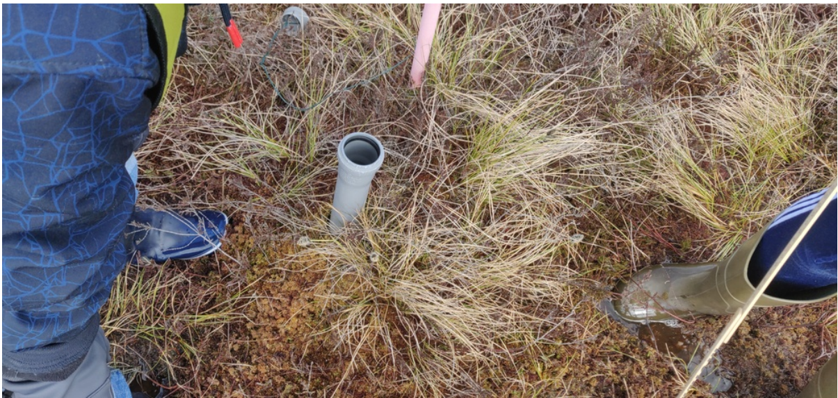
Figure A11: Example of a well where the loggers are located
