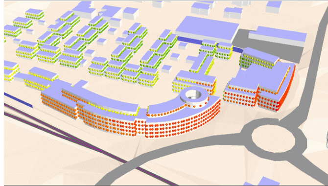
Figure 4.6 - 3D building model showing that it is possible to define noise receivers on different floors of the building using a 3D noise model (SoundPLAN, 2020).
