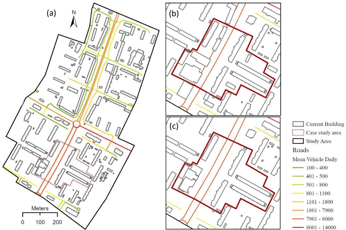
Figure 4.4 - road traffic load pattern. the average number of vehicles in 24 hours passing through on weekdays in 2020 (a) illustrates the whole study area, while (b) displays the planned and current buildings (scenario 1) and (c) displays just current buildings (scenario 2) and their proximity to roads in the case study area. In scenario 1, there are a few planned buildings that intersect with the existing roads. The proposed plan involves modifying the road layout to accommodate these buildings.
