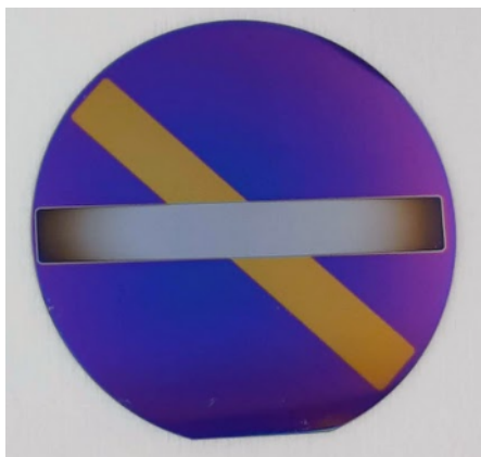
Figure 2.2: Silicon wafer coated with PMMA having two rectangular stripes after argon milling, 4 minutes of milling on the horizontal stripe, and 1 min of milling on the other.
