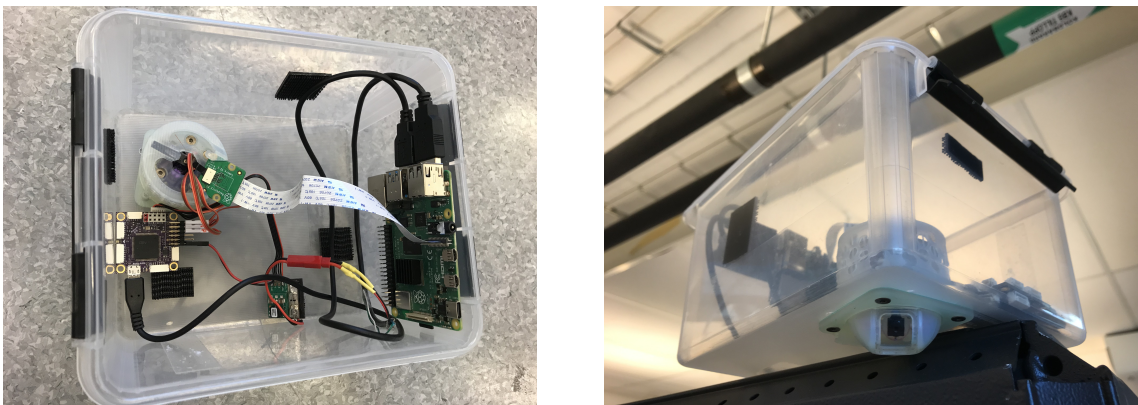
Figure 3.1: Pictures of the box that houses the drone hardware for the experiment. The left picture shows the box from above, from the left the following components are visible: a flight controller, a gimbal with a camera module, a power supply module and a Raspberry Pi. The right image shows the box from below.
