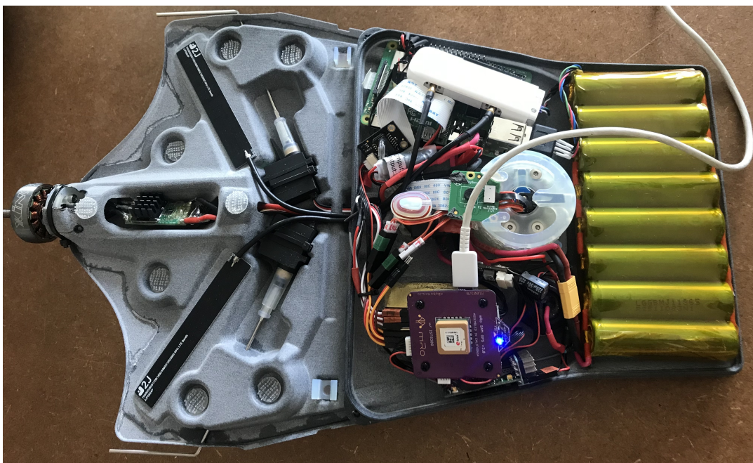
Figure 2.3: The housing of the drone’s components. On the left side, the motor, antennas and control surface servos are visible. In the housing to the right, from top to bottom: RPi with a 4G modem on top, gimbal, GPS module and flight controller mounted beneath it. To the right, the battery pack can be seen.
