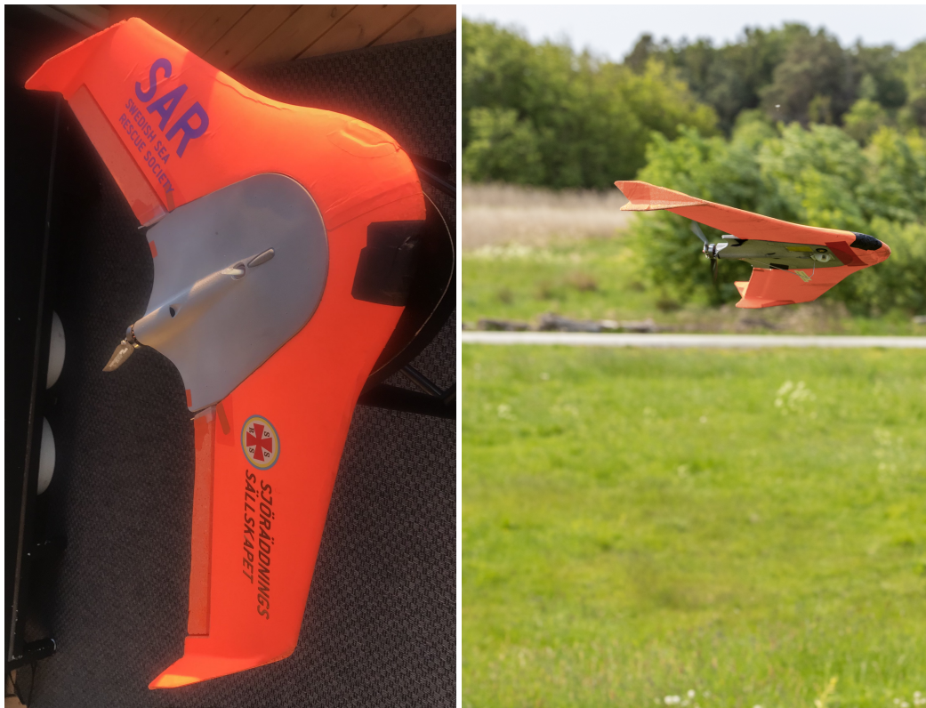
Figure 2.1: The SSRS fixed-wing drone. The left picture shows the drone from above. In the right picture, the drone is seen in flight with the gimbal and camera visible. Right picture credits: Mats Ryde.
