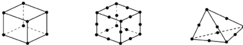
Figure 19: Types of Geometric Order, Linear, Quadratic and Modified Second Order, Hibbitt et al. (2011)
