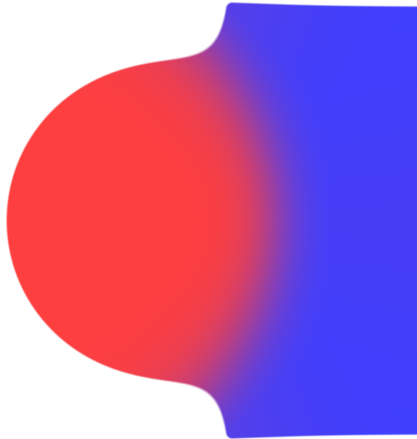
Figure 4.6: A smooth union between a circle and a box of different colours
