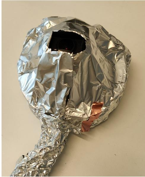
*Figure 3.10: Aluminium foil shield without lens obstruction.*
