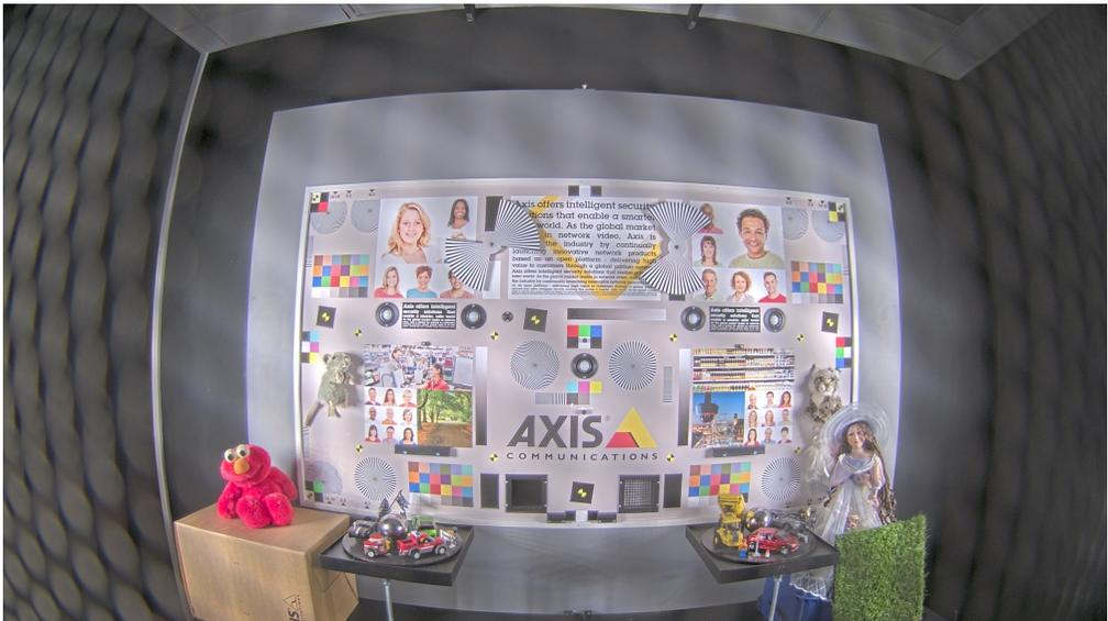
*Figure B.5: Visual light image with aluminium mesh shield attached.*
