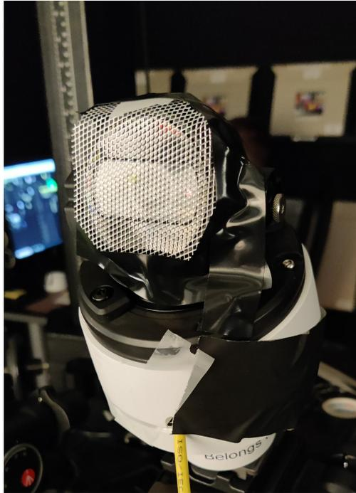
*Figure 3.17: Close up photo on the mounted camera, with the aluminium mesh attached to the lens.*
