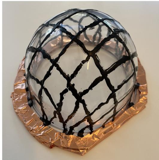
*Figure 3.8: Ink mesh prototype shield coated on a camera dome, copper tape for galvanic connection.*
