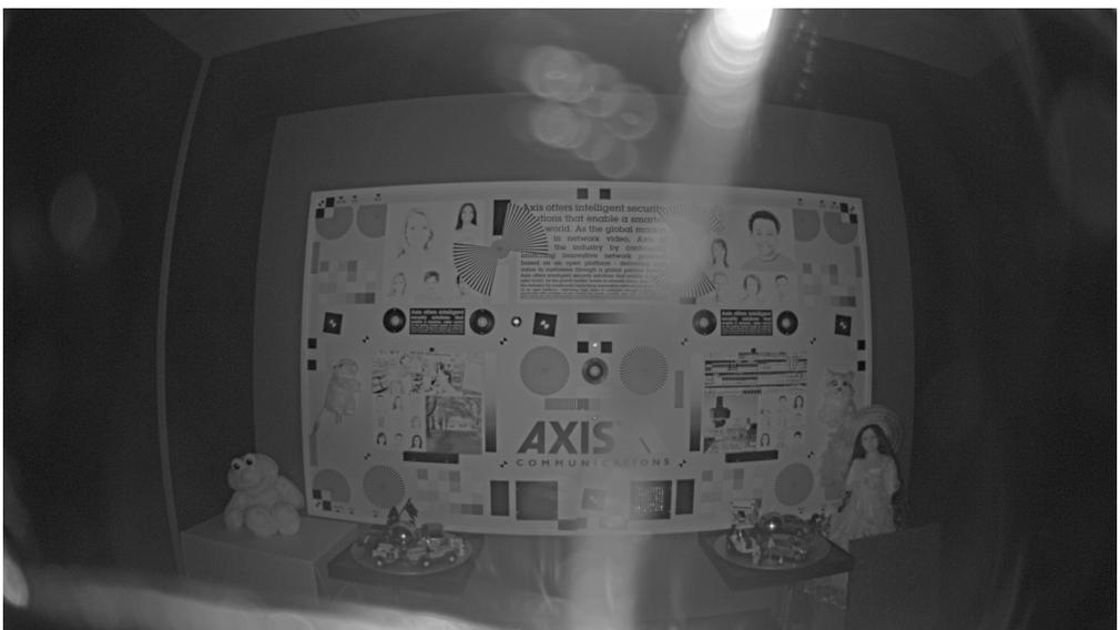
*Figure B.9: Infrared light image with galvanized mesh shield attached.*
