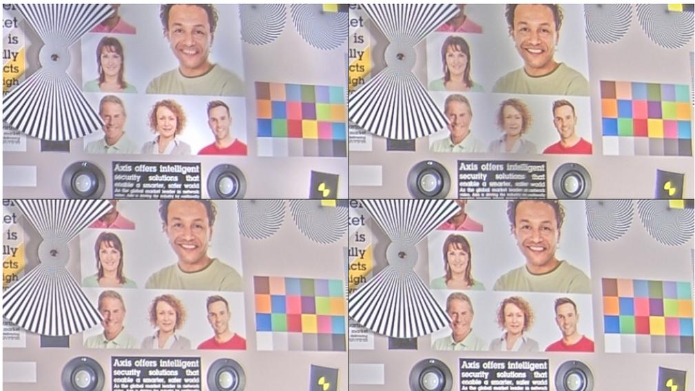
Figure 4.27: Zoomed in image test with four shields. Starting upper left corner and moving clockwise: aluminium mesh, galvanized mesh, silver film and ITO film.
