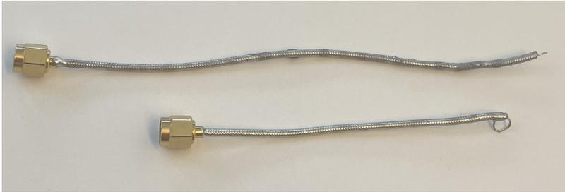
*Figure 3.11: Two near field probes constructed by us. The above one is an E-field and the bottom one with the loop is the H-field probe.*
