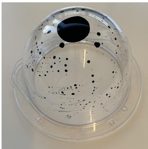
*Figure 3.9: PEDOT:PSS prototype shield painted on a camera dome.*
