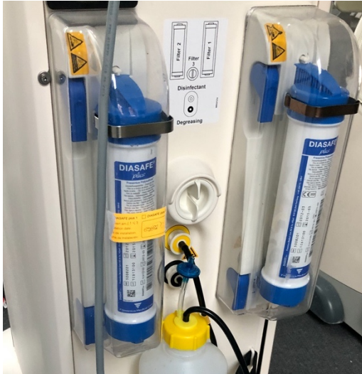
Fig. 8. Filters located on the back of the HD machine. They are changed every third month.
