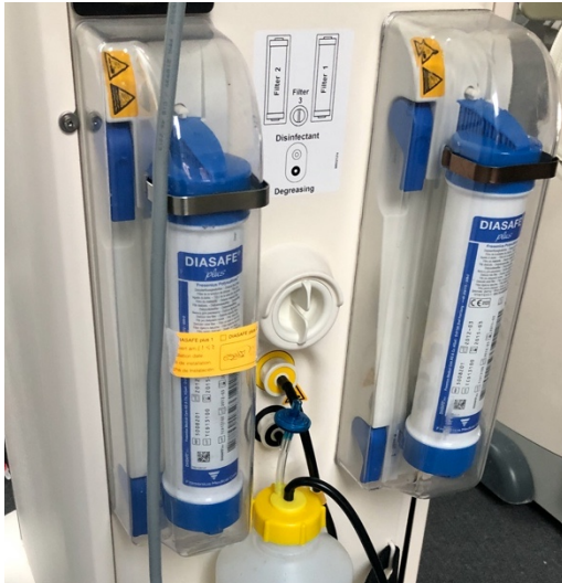
Fig. C2. Filters located on the back of the HD machine. They are changed every third month.
