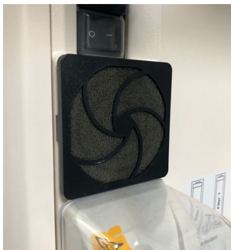
Fig. 10. Image showing the fan that needs to be cleaned from dust every now and then.
