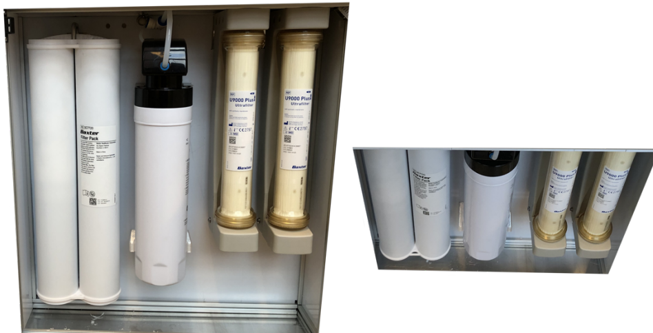
Fig. 15. Two images showing the physical interface for water consumables in the device with filters from left to right: Filterpack, DRO and Ultrafilters. The left picture is taken when bending down, the right one is taken from eye height, sitting.
