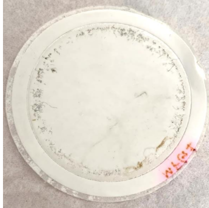
Figure B3. Picture of MFG1 after the parameter study, where visible matter is present on the filtration area.
