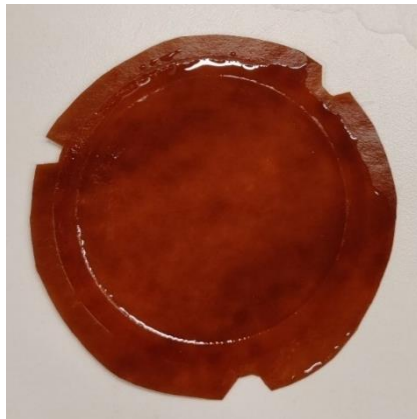
Figure D4. Membrane after filtering LU step 2 process water, the second try. The stirrer was secured prior to this run, and a scratched circle is not visible on the membrane.
