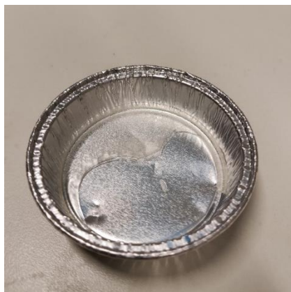
Figure D5. Retentate from Tetra Pak step 2 dried, creating a film.
