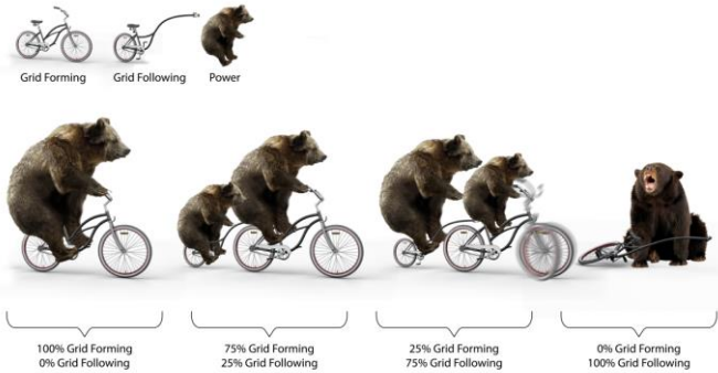
Figure 4-21 Illustration of the issues underlying the stability of the network. The size of the bear corresponds to the power level. Grid forming can correspond to a SG or an IBR operating with grid-forming control. A high proportion of grid-following can lead to instabilities (Kenyon, Hoke, et al., 2020).
