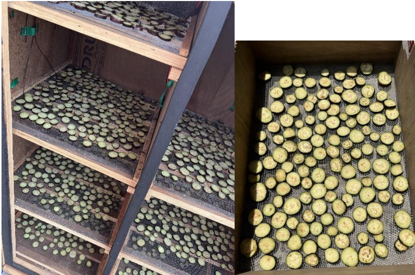
Figure 3. The left image shows two kilograms of eggplants sliced thinly and homogeneously. The slices were then arranged and deposited in every tray of the solar dryer. The right image displays a single tray of sliced eggplants.
