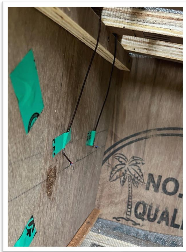
Figure 2. There is a thermocouple with a soldered tip placed in the solar dryer chamber.
