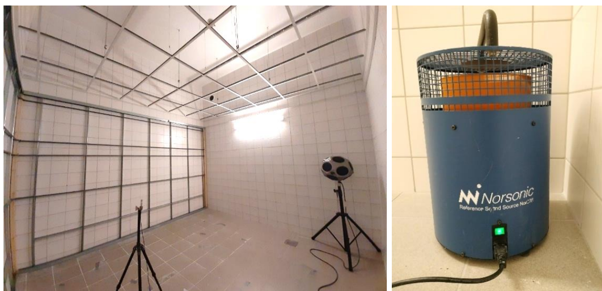
Figure 3-7. Left: Microphone and loudspeaker set up in the reverberant room. Right: Reference sound source for measurement of sound strength G.
