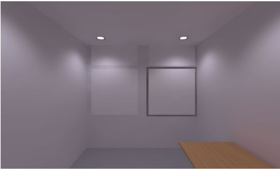
Figure 8: DIALux rendering of 77447 Pleiad Evo's light distribution in the test room.
