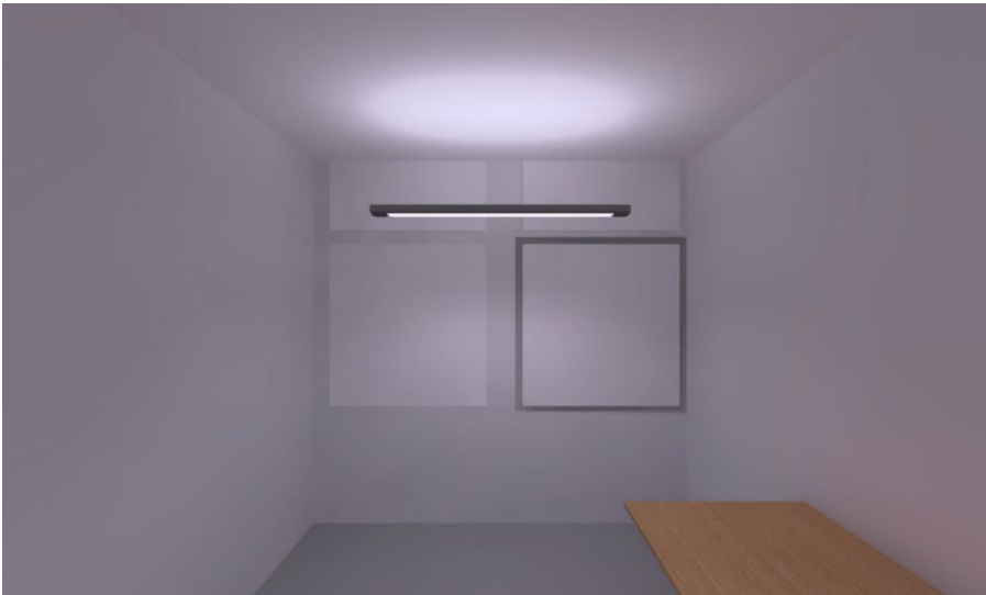
Figure 9: DIALux rendering of 29475-402 DTI LED Type 2's light distribution in the test room.
