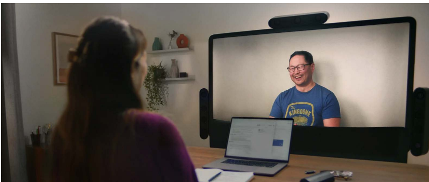
Google's Project Starline utilizes a complete setup of cameras to capture users and a 3D screen to display them. Only one person can be in front of the display, as the cameras use head-tracking to simulate a 3D image on-screen.
