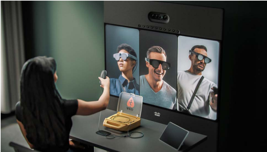
Cisco's system uses a camera booth to capture users, and Magic Leap's AR glasses to display users as holograms. The booths are meant for single-person use.
