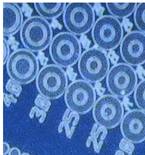
Figure 3.1: Picture of fabricated capacitor rings. The numbering refers to the diameter of the inner capacitor circle in \mu\text{m} .
