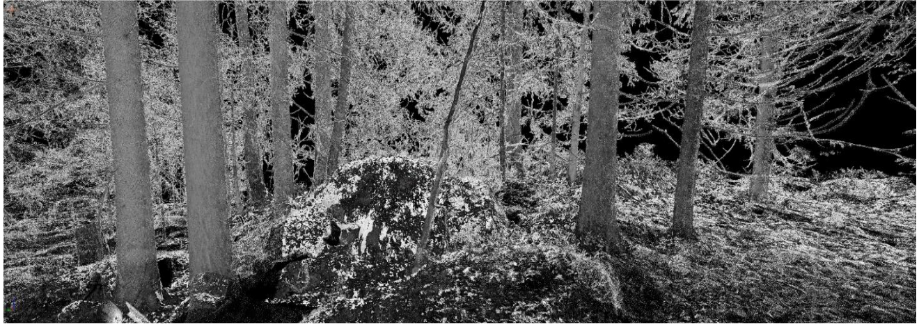
Figure 3. Image of the 3D-model showing the centre of the scanned plot in Rumperöd when processed in RiSCAN. The point cloud was later further processed by TreeLS in R.
