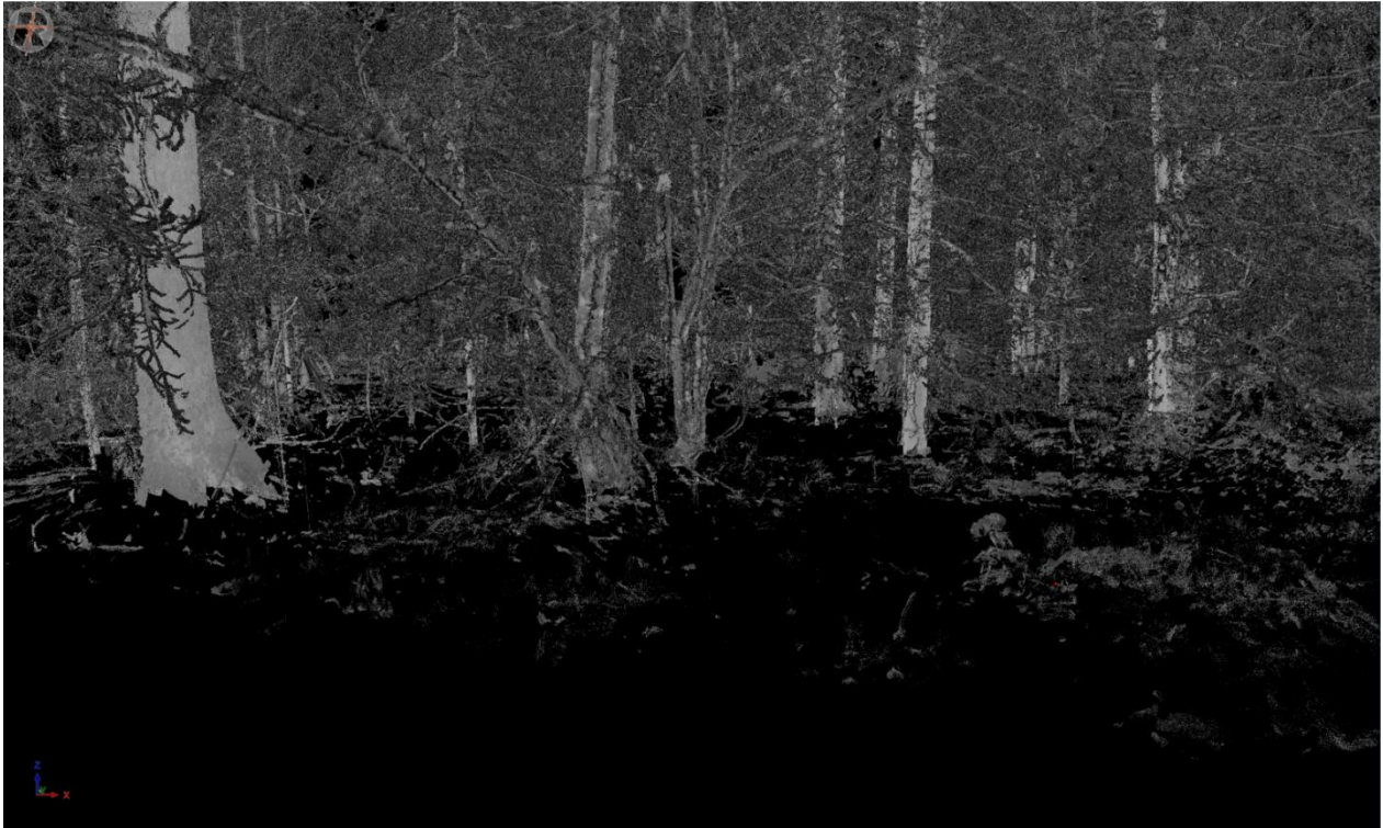
Figure 6. The normalized point cloud with the irregularities of the terrain flattened out when inspected in RiSCAN.
