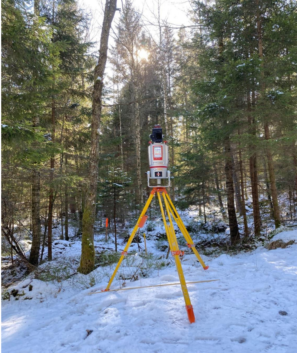
Figure 2. Terrestrial laser scanner RIEGL VZ 400i in the field mounted on a tripod during a test run in Rumperöd, these measurements were not used in the study due to the snow conditions. The red pole in the background marks the center of one of the scanned plots.
