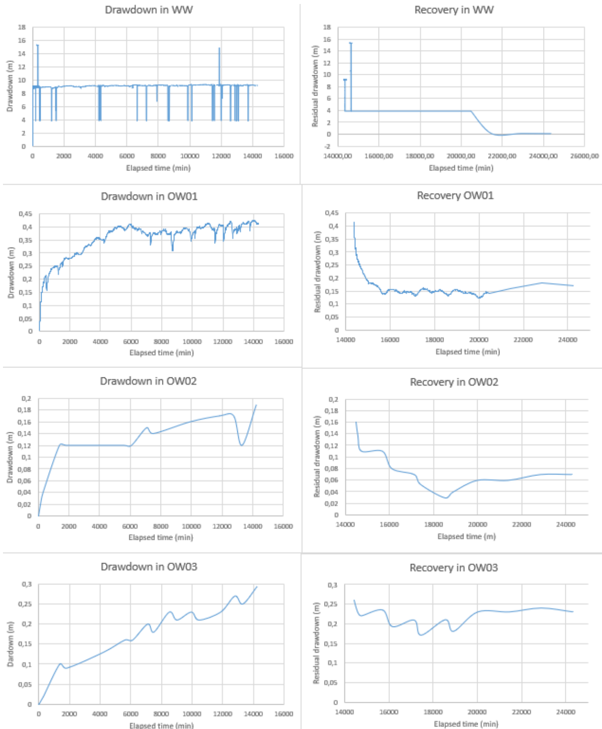
Figure 15: Drawdown and recovery data in all the wells. The raw data for WW and OW01 is obtained by divers.
