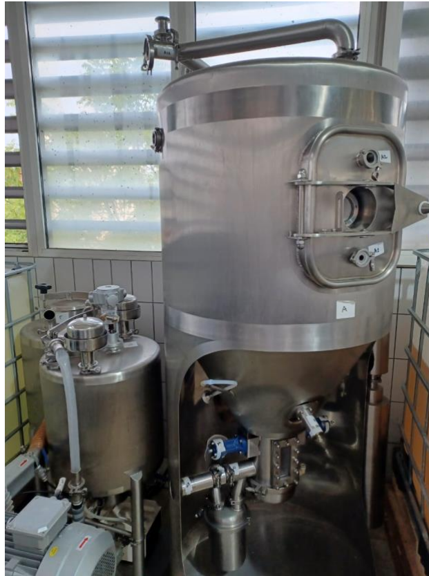
Figure 21: Laboratory scale spray dryer with a capacity of powder yield up to 5 kg/h.
