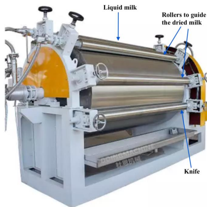
Figure 2: Drum dryer. Commercial product (5)
