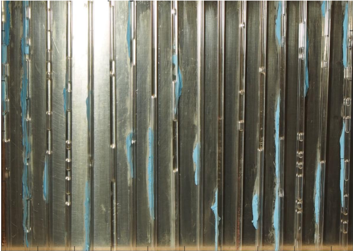
Figure 27 Visualization of the chaotic flow and different flow patterns in the adiabatic section of the PHP when in operation.
