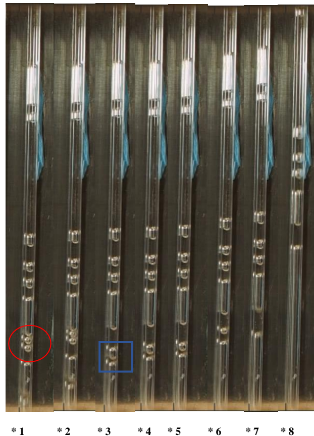
Figure 28 Flow pattern development in a single channel of the PHP.
