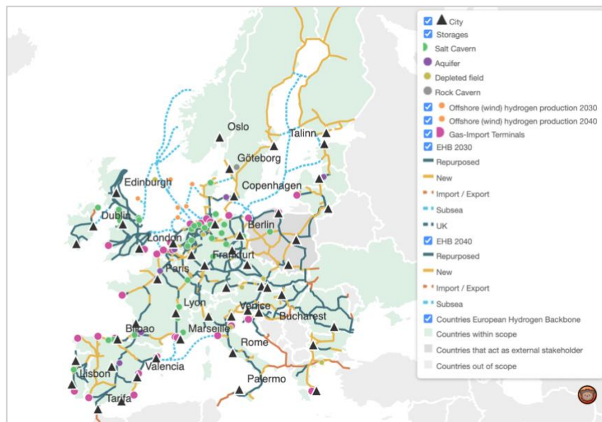
Figure 1: Map of the European Hydrogen Backbone and the envisioned infrastructure up to 2040 1
