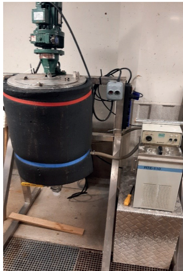
Figure 9. Stirred heated tank for 24 hours KGM preparation.
