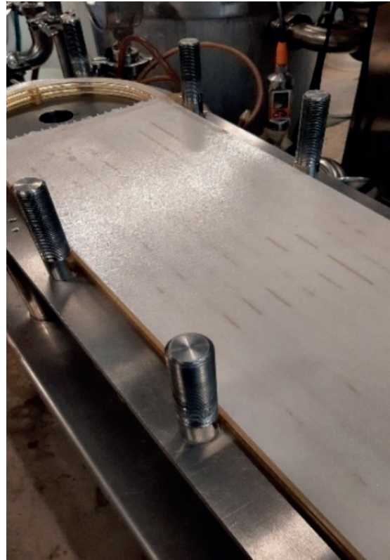
Figure 5. RC70PP membrane installed in the M39 module.
