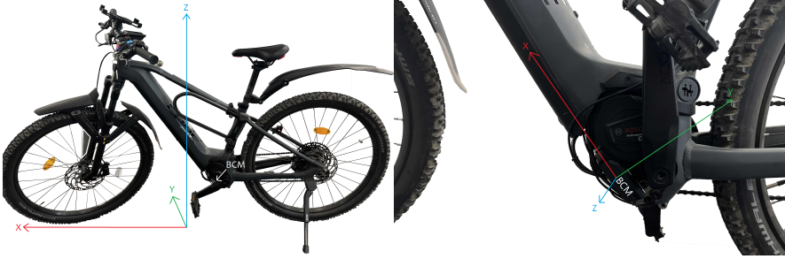
Figure 3.1 The eBike's coordinate frame visualized. Figure 3.2 The mounted BCM's coordinate frame visualized.
