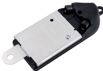
Figure 2.2 The bcm3 unit containing a GNSS as well as an IMU.
