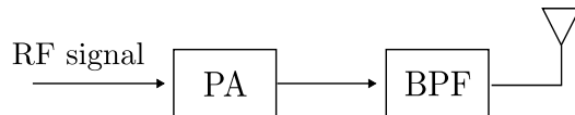
Figure 2.2: The structure of an ET consisting of a single RF chain with a single antenna, the PA block is the power amplifier and the BPF block is the bandpass filter.
