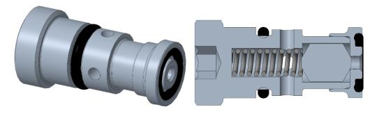
Initially the value is forced closed by a spring which prevents leakage. When the oil pressure (in the right side of the image) reaches a certain point, it will overcome the spring and transfer the cylindrical pin to the other side. Conversely, it will return to its original position when the spring overcomes the oil pressure on the other side. It is this small movement back and forth that allows air to escape past the small pin while keeping oil inside.
