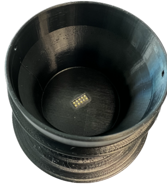
Figure 4.17 Pogo pins inserted in the bottom of the holder.
