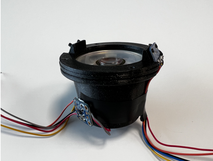
Figure 4.36 The speaker box together with the speaker and the speaker clamp with microphones installed on the clamp. The amplifier is mounted on the speaker box.
