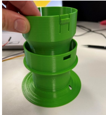
Figure 4.6 3D-printed model for testing snap fits.
