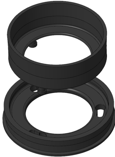
Figure 4.5 CAD-model showing the fastening concept using bayonet mount.
