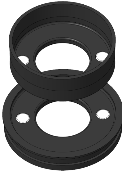
Figure 4.4 CAD-model showing the fastening concept using magnets.
