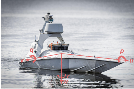
Figure 3.1 Figure showing the 6 DOF of a marine ship; surge u , sway v and heave w and angular velocities p , q , and r . Photo: Saab Kockums / Glenn Pettersson.
