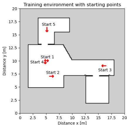
Figure 3.4 Map of the training environment with the five starting points (red arrows) used during data generation. The black lines are walls, the white areas are inside the building and the grey areas are outside. Only goal points in the white areas are viable.
