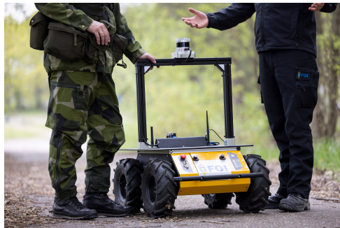
Figure 3.1 The UGV considered in the thesis, the Husky platform equipped with a LiDAR sensor. A simulated version of the Husky is used during data generation and testing.
