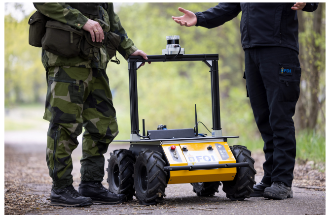
Figure 1. The UGV used in the thesis, the Husky platform from Clearpath Robotics.
