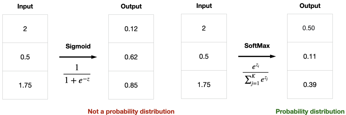
Figure 2.2: To the left is an input vector where the Sigmoid function is applied to create the corresponding output, here the resulting vector does not become a probability distribution. To the right is the same input vector, but here the SoftMax function is used instead. The resulting output vector now becomes a probability distribution where the sum of the vector adds to one.
