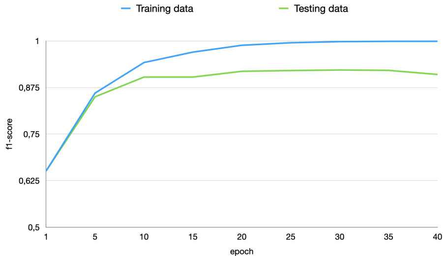
Figure 4.1: The f1-score of the blazintext algorithm when trained for various numbers of epochs. The optimal result is obtained by stopping the training at around 30 epochs.
