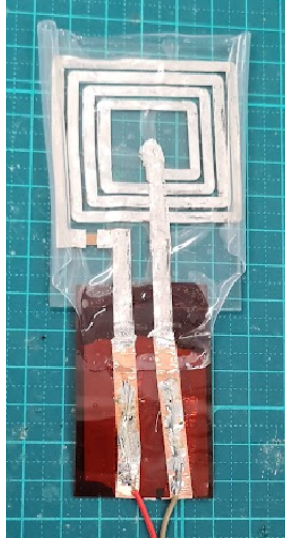
Figure 2.12: Stretchable coil manufactured by Matsuhisa Laboratory.
