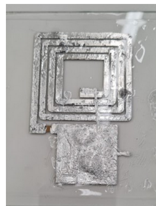
Figure 3.29: Stretchable series RLC sensor, R_{sensor} = 5 \Omega , L_2 = 881 \text{ nH} and C_2 = 1.4 \text{ nF} .
