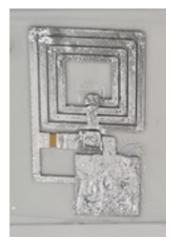
Figure 3.28: Stretchable parallel RLC sensor,  $R_{sensor} = 2 \Omega$ ,  $L_2 = 881$  nH and  $C_2 = 1.4$  nF.
