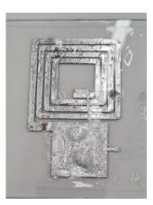
Figure 3.29: Stretchable series RLC sensor,  $R_{sensor} = 5 \Omega$ ,  $L_2 = 881 \text{ nH}$  and  $C_2 = 1.4 \text{ nF}$ .
