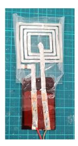
Figure 2.12: Stretchable coil manufactured by Matsuhisa Laboratory.
