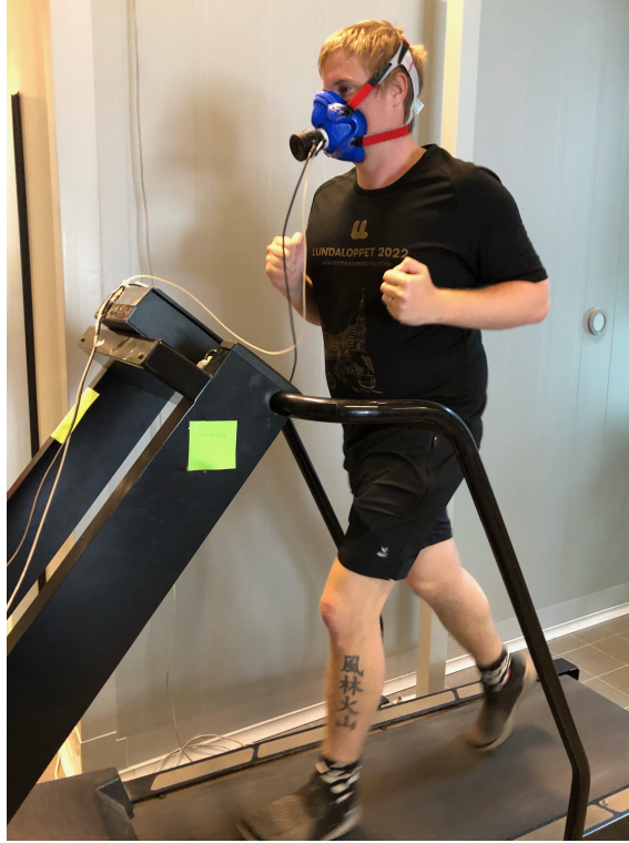
Figure 3.5: Test set up. Subject running on treadmill wearing mask connected to Metamax 3B
