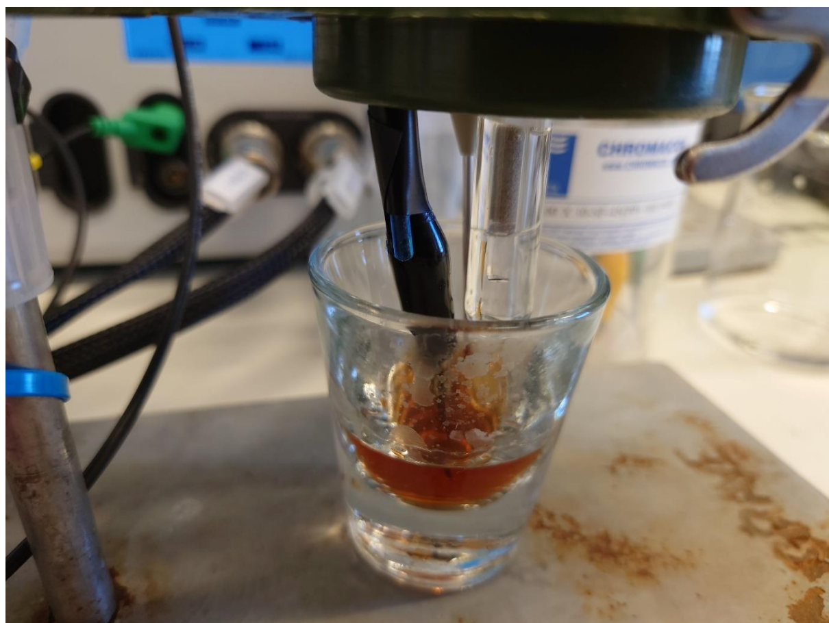
Figure 18: Experimental setup for cyclic voltammetry. In front: crocodile clamp with attached working electrode, right Ag/AgCl reference electrode, in the back is the Pt auxiliary electrode.
