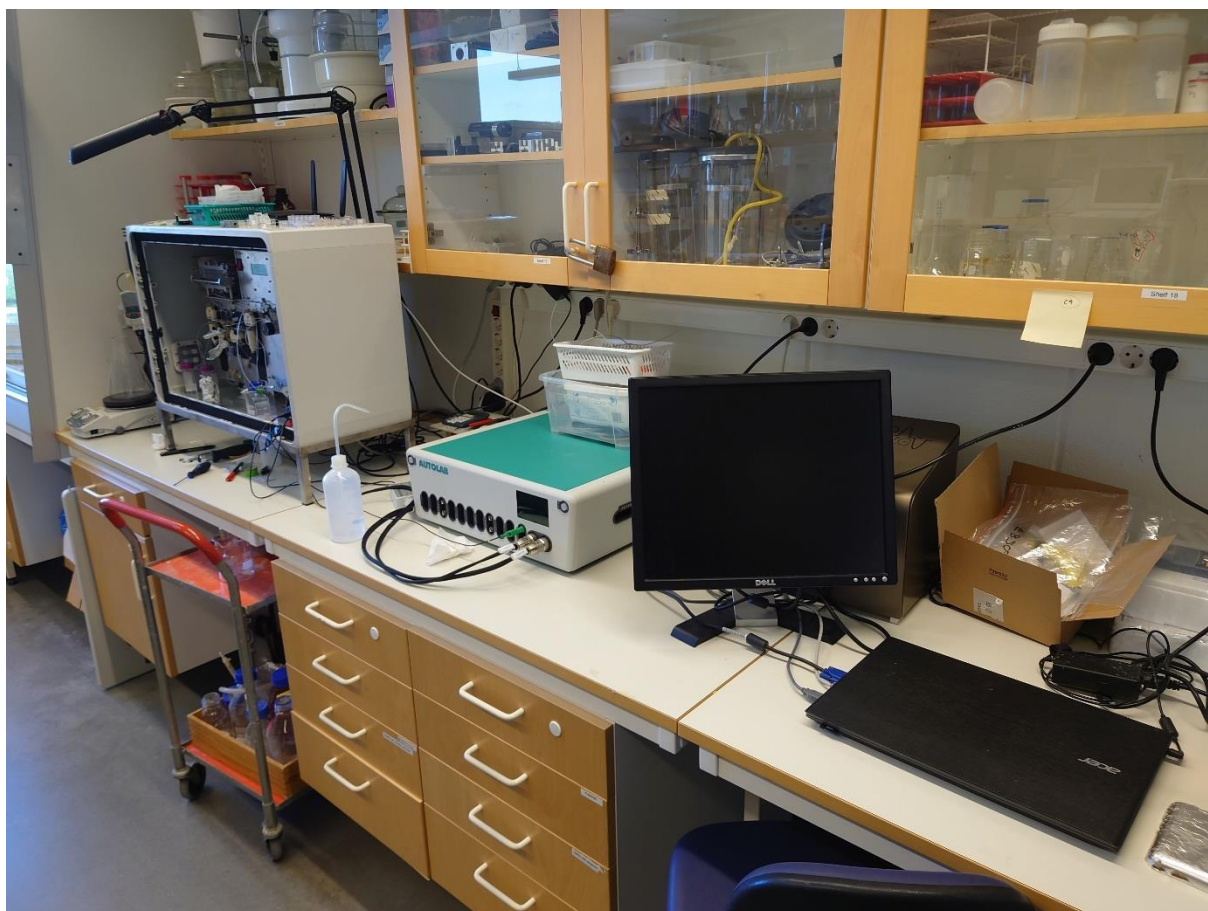
Figure 21: Overview of the final amperometric setup with attached FIA-system. FIA- system to the left, Autolab PGSTAT 302N I the middle and computer control computer to the right.
