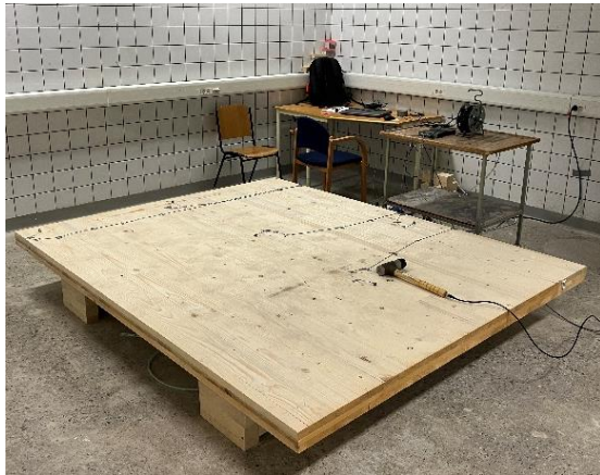
The test setup for measuring the material properties of the CLT-floor panel
