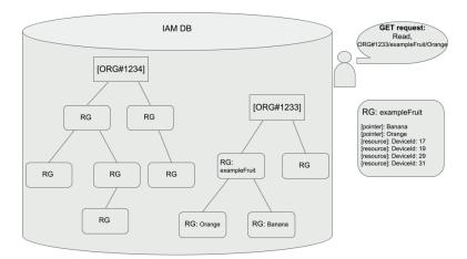
Figure 20: The structure of data in the RG access tree
