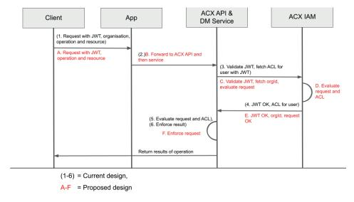
Figure 37: Comparison between current authorisation flow for a request, and the proposed flow
