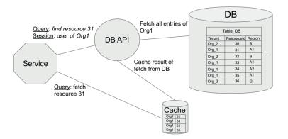
Figure 12: Data storage and querying architecture for the second logical separation case
