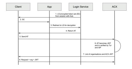
Figure 25: Current authentication in ACX with AT
