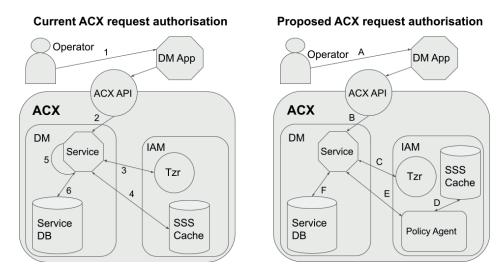
Figure 35: Comparison between current authorisation flow for a request, and the proposed flow
