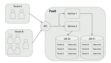
Figure 1: Example of multitenant architecture
