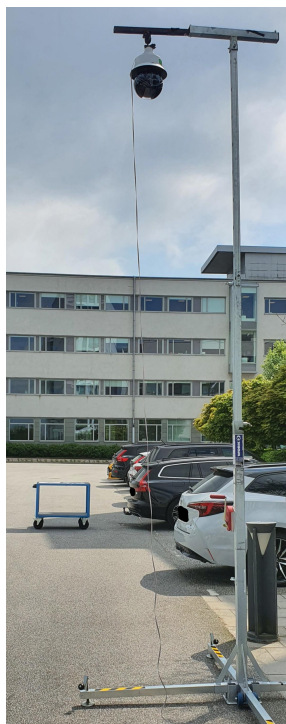
Figure 5.1: Temporary setup for testing the height estimation from the calibration procedure. The two calibration papers are lying on top of the blue table with a height of 1.01m from the ground. The height of the camera stand could be changed between measurement tests.
