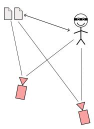
A movable camera, also called a PTZ camera, uses built-in motors to move around which enables it to see its whole surrounding. The ability to move makes it possible for this kind of camera to follow moving targets in a scene, an action called tracking.
