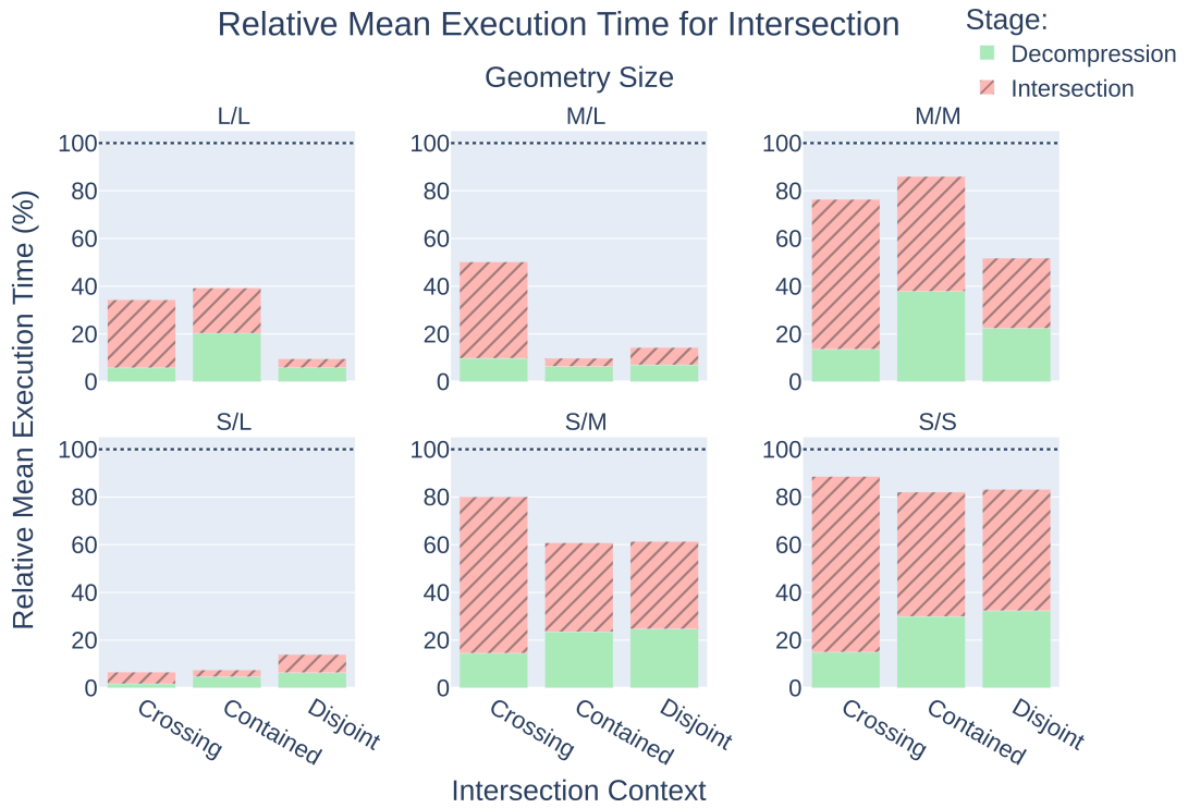
Figure 5.5: Fractions for the relative execution time of the de-compression and the intersection algorithm stage for FPDE.
