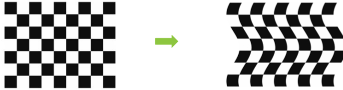
Figure 1.1: Illustration of rolling shutter artifacts. If a camera captures the checkerboard in the left image whilst moving periodically back and forth horizontally, capturing one line at a time from the top down, the resulting image will look similar to the right image
