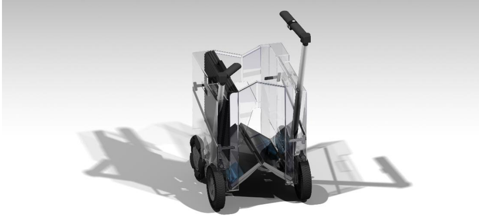
Figure 6.3 Transparent version of the vehicle when semi-folded and with semi-raised handles
