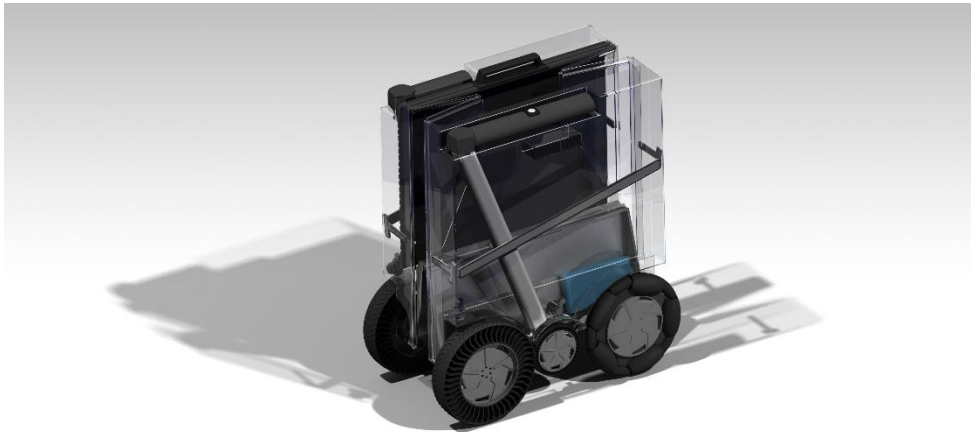
Figure 6.2 Transparent version of the vehicle when folded
