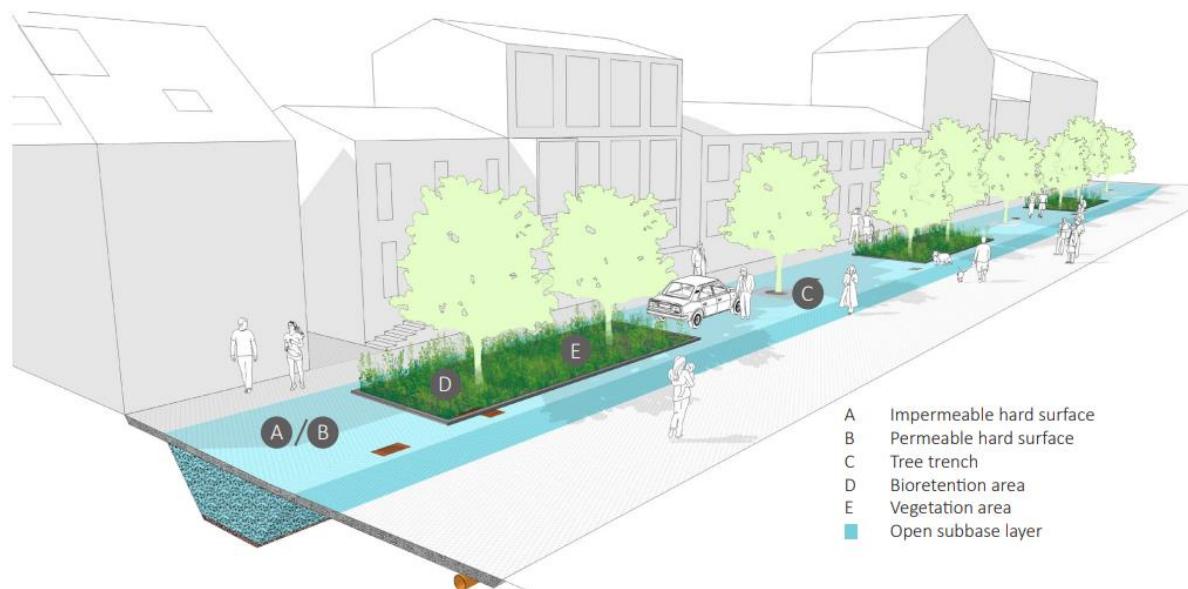
Figure 2.4.3: The concept of the BGG system introduced by EDGES where the crucial infrastructure of a city i.e., roads are included in stormwater management in urban areas. The sub-base layer is replaced with an open subbase layer (OSL) to make rum for retaining water and accommodate bioretention areas or tree trenches together while providing a hard surface on the top to carry traffic loads. In this BGG OSL section is continuous along the long section of the street to maximize the capacity ( Livable-Streets-A-Handbook-of-Bluegreengrey-Systems-Version-2.0.Pdf , 2020)
