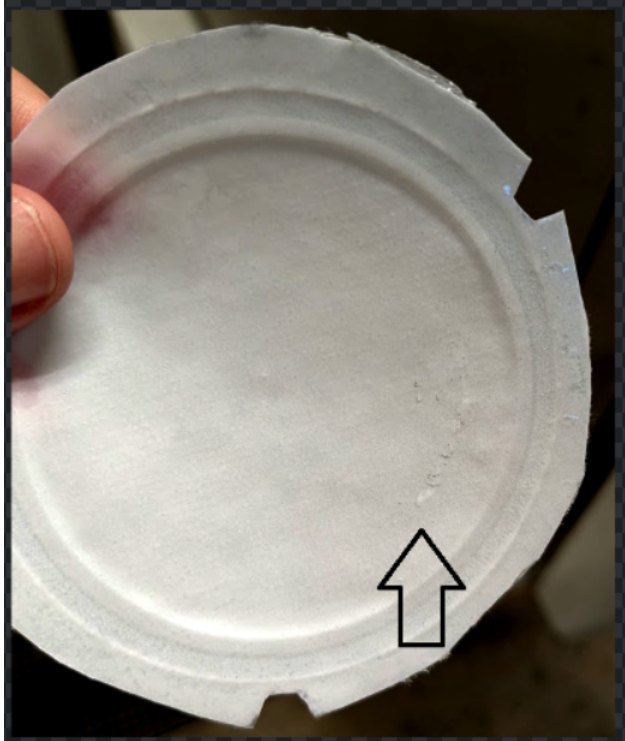
Figure 4.1: Picture of RC70PP membrane after experiments, with arrow pointing to damage
