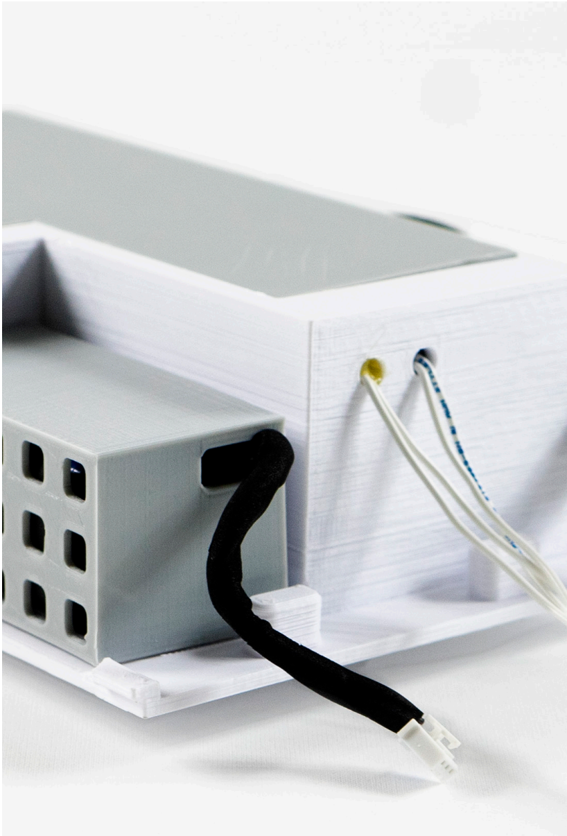
Detail view of battery and driver blocks, back shell removed.
