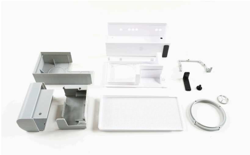
Top: 3D printed parts of BLOK speaker. Right: detail of 3D printed part.
