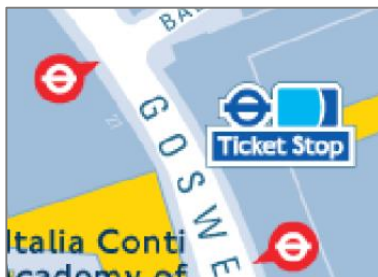
Figure 4: Adjust the position of TicketStop symbol to the pavement. Avoid placing it centered on the point it represents, so the user can easily interpret on which side of the road it is in reality © Copyright Transport for London
