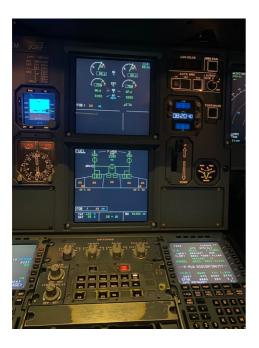
*Momentary Avionics Smoke warning.* When passing approximately FL260 (26 000 feet), a momentary "AVIONICS SMOKE" warning was triggered in the aircraft's ECAM (Electrical Centralised Aircraft Monitor) system. The warning disappeared by itself after approximately three seconds, to allow crew to clearly observe it, but not to take any action or start the associated procedure.
