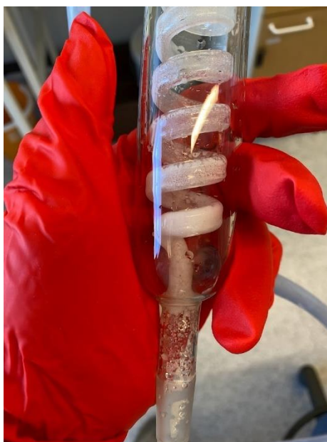
Figure 13 – Precipitation is visible in the gas condenser after the "test 1 - 120 min - 80°C, 1 l/min".
