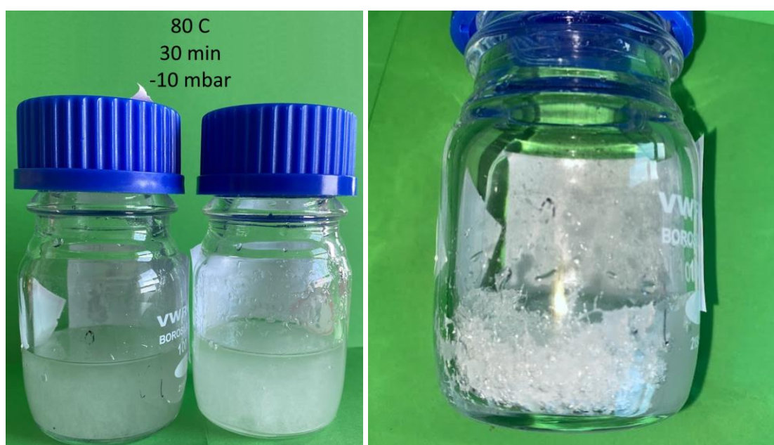
Figure 18 – Pictures of the pilot samples after they had been regenerated at 80°C and -10 mbar for 30 minutes. On the picture on the right, it is possible to see precipitation that looks different than what it does at in the lab. The picture on the right is tilted to show the precipitate more clearly.
