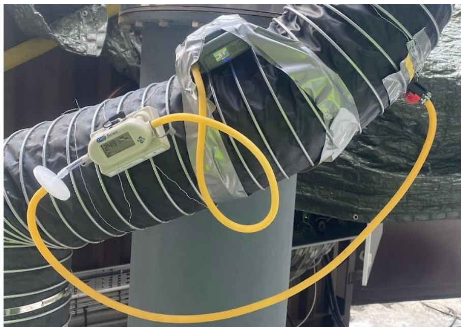
Figure 4 - A picture of the sampling setup at the pilot plant. A Thermosorb-N cartridge is connected to the setup to sample the concentration of nitrosamines at the inlet of flue gases to the absorption tower.
