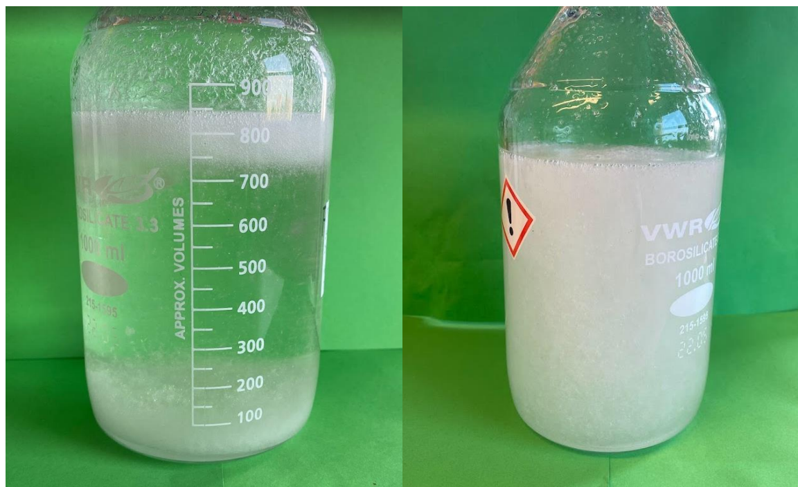
Figure 17 - Sample from the regenerated AMP/DMSO solution taken from the bottom of stripper tank 1 at the pilot plant. The sample in the picture on the right had been shaken prior to the photograph to visualise how the sample would look at the pilot plant under agitation.
