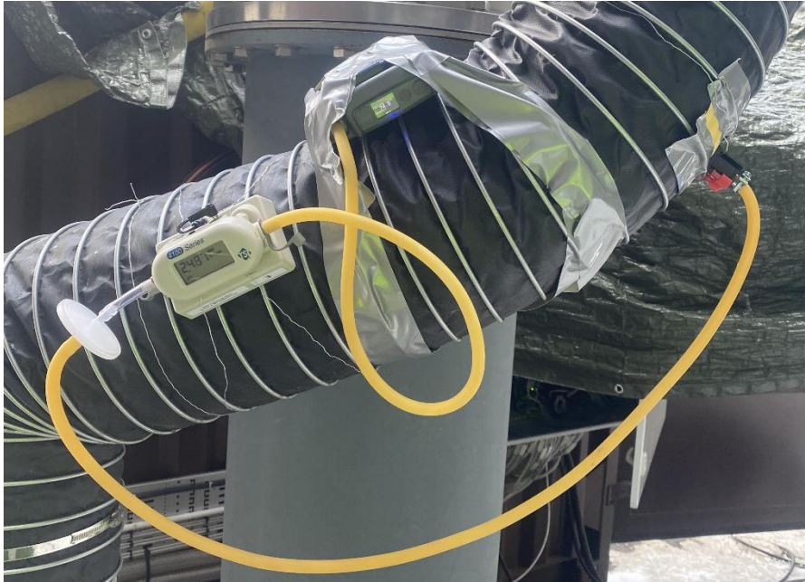
Figure 33 - A picture of the adsorption setup in use at the inlet of flue gases to the absorption tower.
