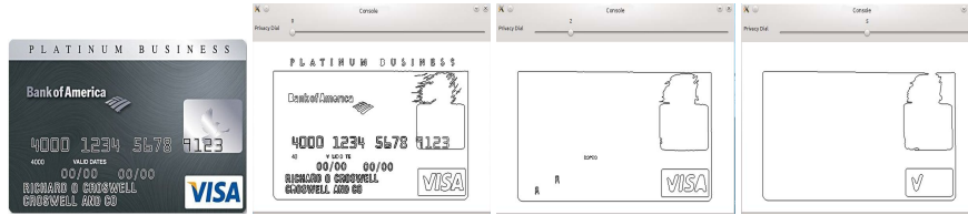
Figure 5.2: Example of the possible outputs of applying sketching transform on a credit card image [59].
