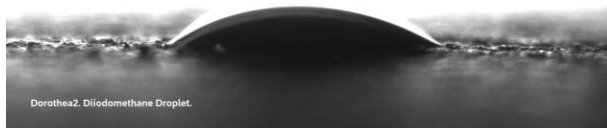
Figure A6 - Drop test on coating: 15 min STEX + MWL, diiodomethane droplet, water picture missing
