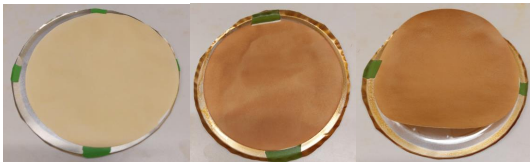
Figure A2 - Filter paper with lignin coatings. Samples left to right: STEX 5 min + enzymatic hydrolysis + MWL, STEX 15 min + MWL, STEX 15 min + enzymatic hydrolysis + MWL.
