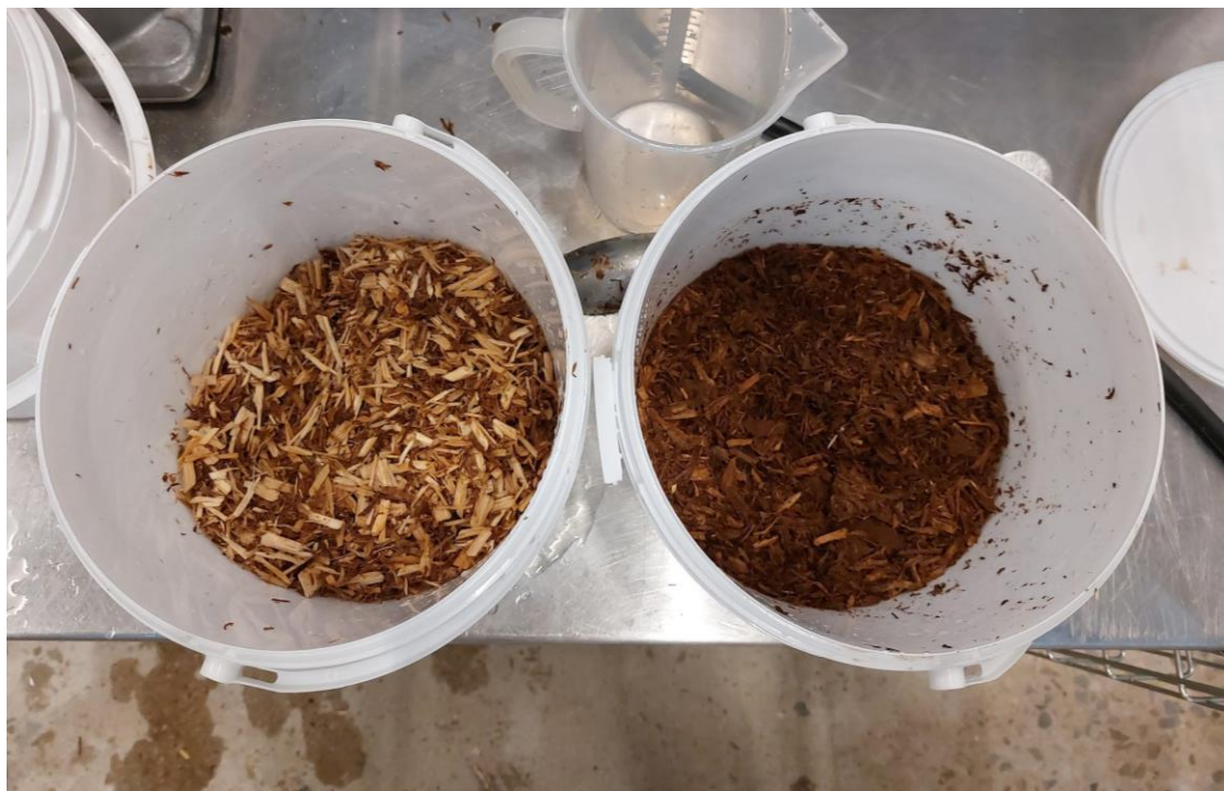
Figure A1 - Biomass after steam explosion. Samples left to right: STEX 5 min, STEX 15 min.
